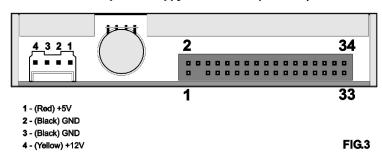
Plug the other end of the short 4-lead colored power supply cable in 3.5" HD floppy drive's 4-pin power supply header. Alternatively, connect external ATX power supply's floppy drive lead to the 3.5" HD floppy drive's 4-pin power supply header if your Apple II cannot deliver enough power for the floppy drive.
